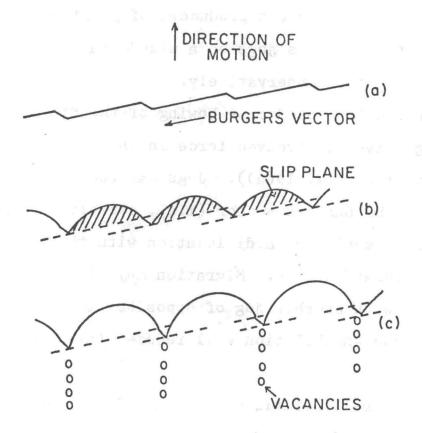
Fig. 12. Motion of a jogged screw dislocation. (a) Straight dislocation under zero stress. (b) Dislocation bowed out in the slip plane between jogs due to applied shear stress. (c) Motion of dislocation after reaching critical stress, leaving trails of vacancies behind the jogs. (After Hull (1965).)
